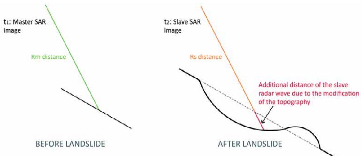
Figure 5: the ground displacement, as a landslide, influences the phase shift of a Radar returned signal. The way of the signal on the Slave SAR image is longer than the way of the signal on the Master image, due to the displacement created by the rotational landslide. This additional distance produces a phase shift that can be detected and interpreted as an active area on susceptibility maps (SafeLand deliverable 4.1).
