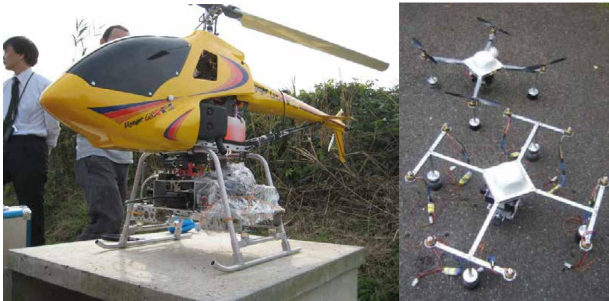
Figure 3: Exemplary light-weight UAV systems. Right: Voyager G8 RR ( http://www.sensor-asia.net/wp-content/uploads/2010/12/IMG_1389.jpg ) , Left: Open-Source multicopter systems [Niethammer et al., 2009]
