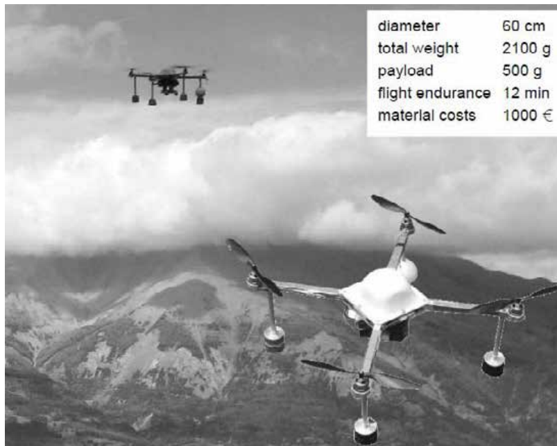
Figure 1: Quad-rotor system for remote-sensing and its main characteristics.
