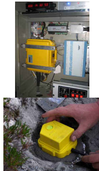
Fig. 4. Up: Data acquisition system of geophone network installed in the upper bunker. Down: Installation of a 3-component geophone.
