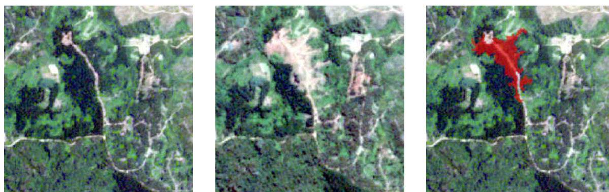
Figure 10 : Multitemporal imagery from RapidEye capturing surfaces changes during the Chilean earthquake 2010. Left: Forested region with steep slope in proximity to Constitución (2010-01-22), Middle: Same scene after the Chilean earthquake 2010-02-27 (hours after the event) showing exposures of bare soil due to landsliding, Right: Results change detection. Source: http://www.rapideye.de/upload/documents/Press_Releases/ChangeDetection_Chile-Earth-Quake_2010-03-04.pdf
