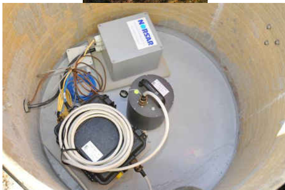
Fig.5. Up: Installation of the broadband seismic station AKN. Down: Seismometer pit with sensor, power/communication module and data acquisition module.
