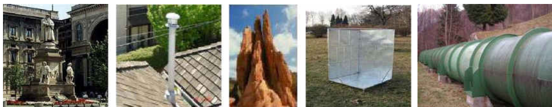
Figure 73 : Examples of man-made structures and stable natural scatterers that return stable signals back to the satellite ( http://www.treuropa.com ).
