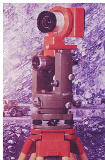
Fig. 3. Wild P32 camera for terrestrial photogrammetry over a theodolite.
