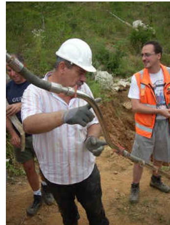
Fig. 10. The deformed module of D.M.S. column showing the displacement of about 60 cm.
