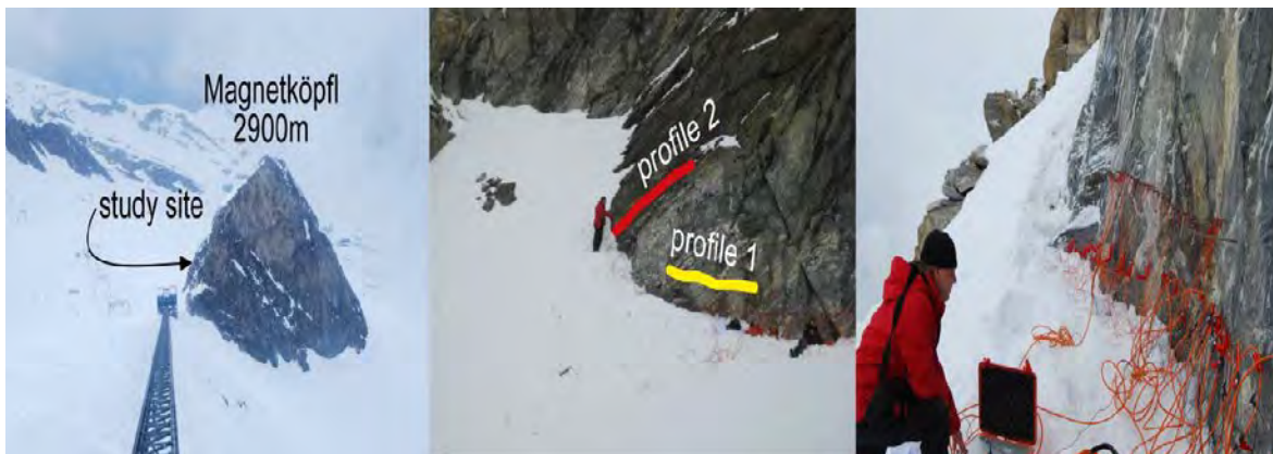
Fig. 2: ERT measurements at two profiles on a rock wall at the Magnetköpfl (Kitzsteinhorn).
