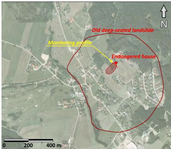
Fig. 5: Orthophoto with the marked landslides and geoelectric monitoring profile. Source of map: GoogleEarth.
