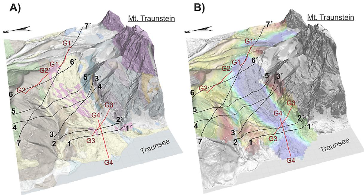
**Fig. 9.** 3-D view of the geological (A) and electromagnetic (B) map seen from the west; black lines: locations of the HEM cross sections; red lines: locations of the geoelectric profiles.
