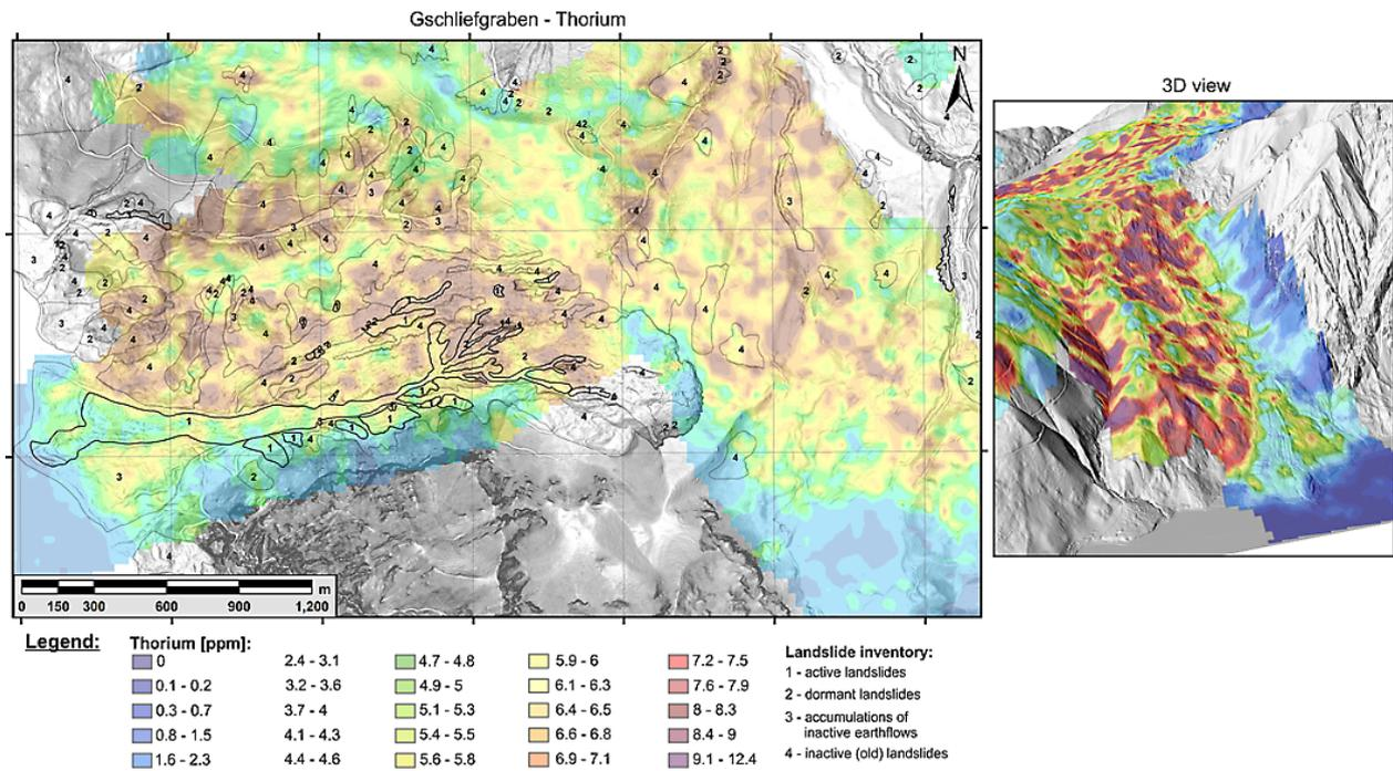
Fig. 12. Map of the thorium content at the ground surface compared to the landslide inventory map; right side: 3-D view from the west.
