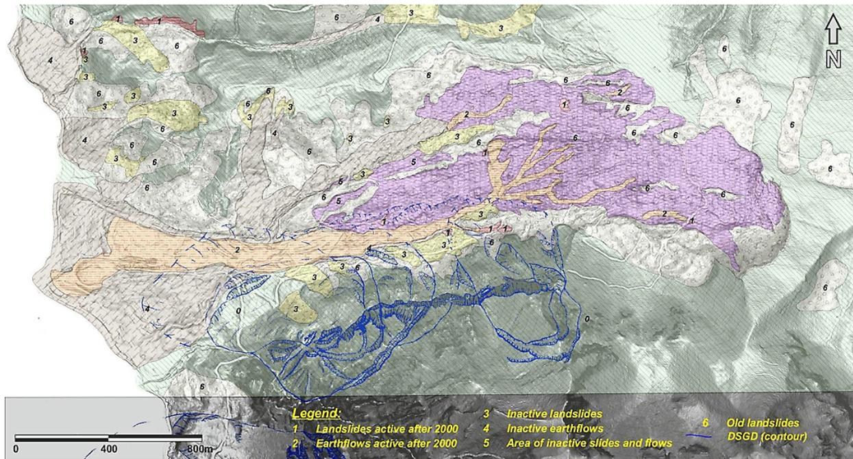
Fig. 4. Landslide inventory map of the area of Gschlieflgraben. Slope failures comprise more than 50 % of the area.
