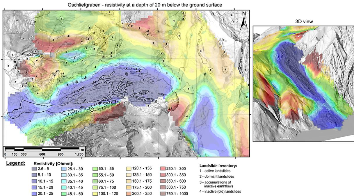
**Fig. 7.** Map of the subsurface resistivity derived from AEM data (depth slice) at a depth of 20 m below the ground surface compared to the landslide inventory map; right side: 3-D view from the west.
