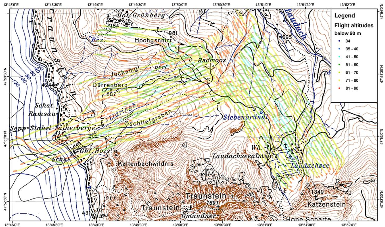
Fig. 5. Flight lines of the Gschlieflgraben airborne survey; colours indicate the actual sensor height (m) above topography.
