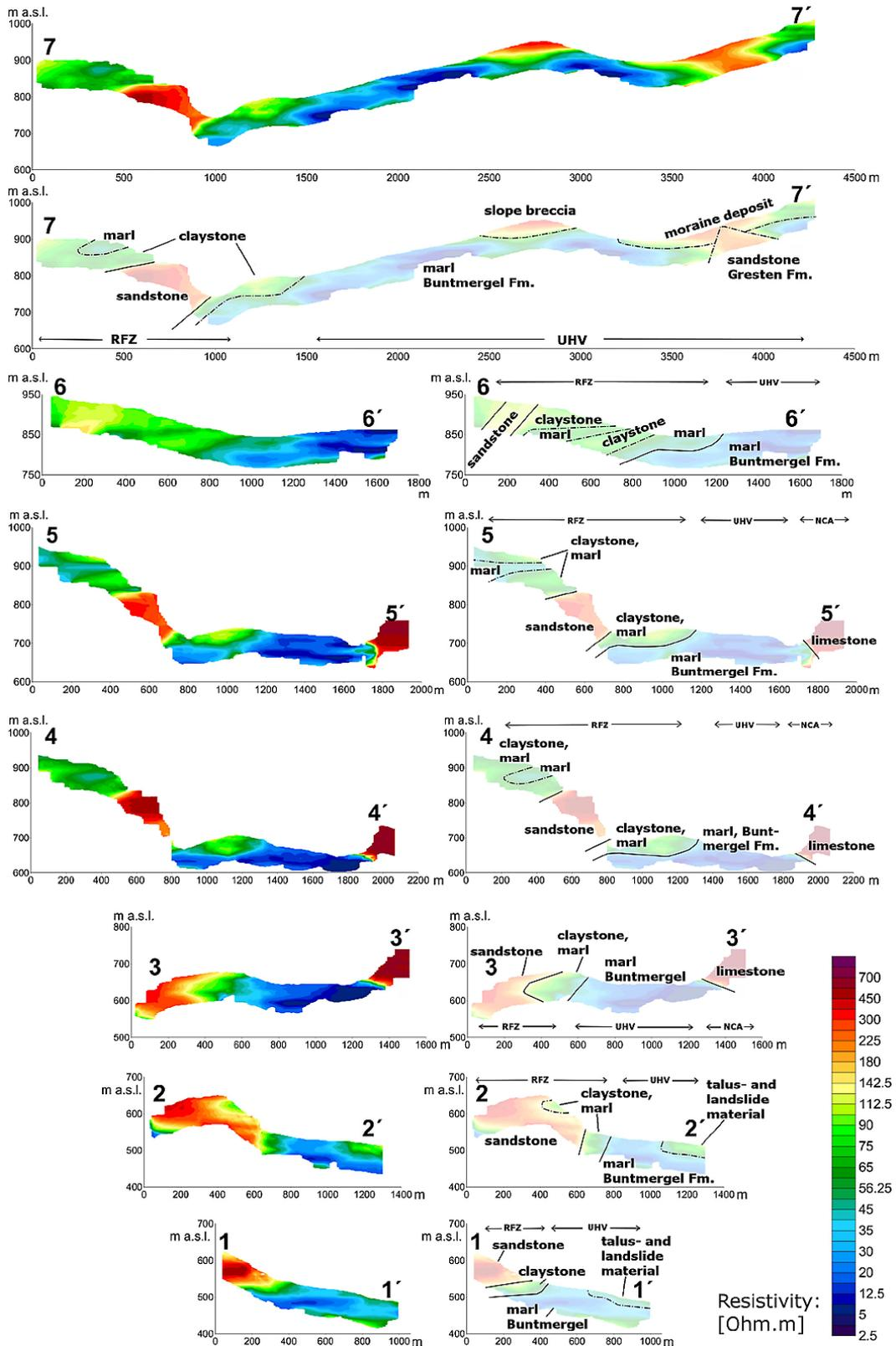
**Fig. 8.** HEM cross sections obtained from the 1-D multilayer inversions; their positions are marked in Fig. 9 (black lines); HEM cross sections with lower colour contrast include geological information for a detailed interpretation of the derived resistivity pattern.
