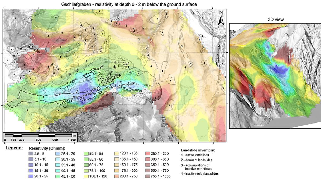
**Fig. 6.** Map of the subsurface resistivity derived from AEM data (depth slice) at depth 0–2 m below the ground surface compared to the landslide inventory map; right side: 3-D view from the west.
