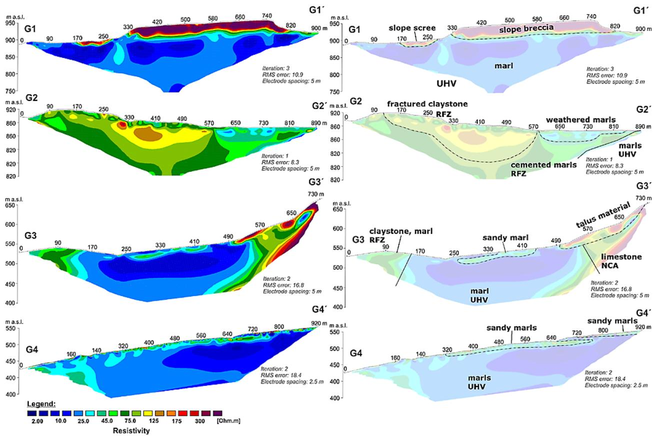
**Fig. 10.** Inversion results of geoelectrical multi-electrode profiles (left), results with low colour contrast including geological information (right); for location see Fig. 9 (red lines, profiles G1–G4).
