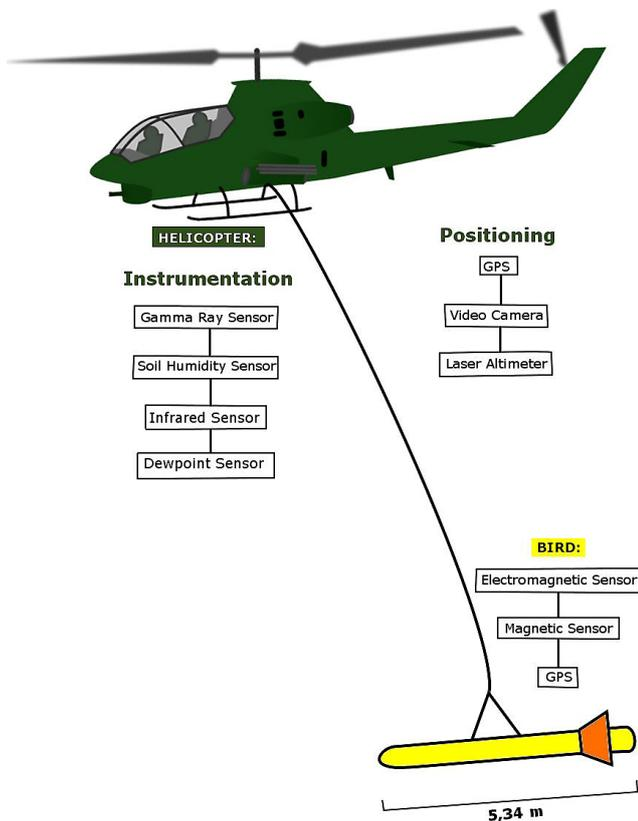
**Fig. 2.** Components of the Austrian airborne system.
