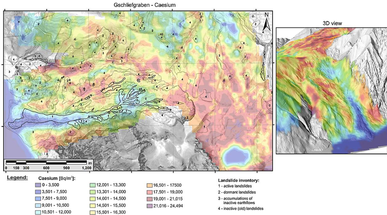
Fig. 13. Map of the Cs activity compared to the landslide inventory map; right side: 3-D view from the west.
