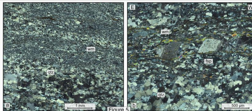
**Thin section observations** revealed that samples from the **Pretul Orthogneiss** consist of quartz, sericitized feldspar, white mica, and rarely observed biotite, which is often chloritized. Accessory minerals are zircon and apatite. Commonly quartz veins crosscut the orthogneiss.
