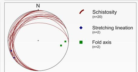
Fig. 6: The bedding of the lithologies show a uniform shallow dip of 20°-30° to WNW. Some outcrops of the orthogneiss show a well-developed lineation dipping shallowly to the SW at 10°-15°. Rarely folds with a shallow E-directed dip are present.
