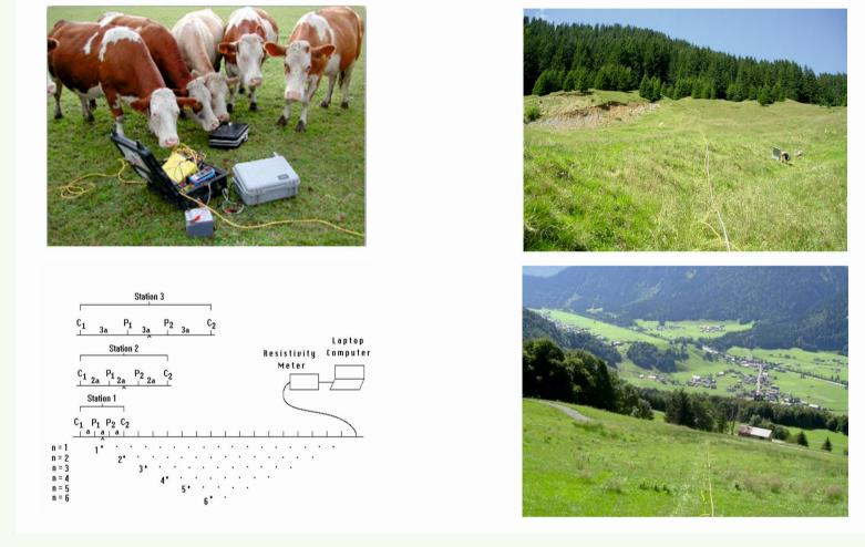
Different materials have characteristic electr. resistivity, ranging from very low (clay) to very high (hard rock), depending also from water content. Electrical resistivity tomography (ERT) is a geophysical technique for imaging sub-surface structures from electrical resistivity measurements made at the surface.
