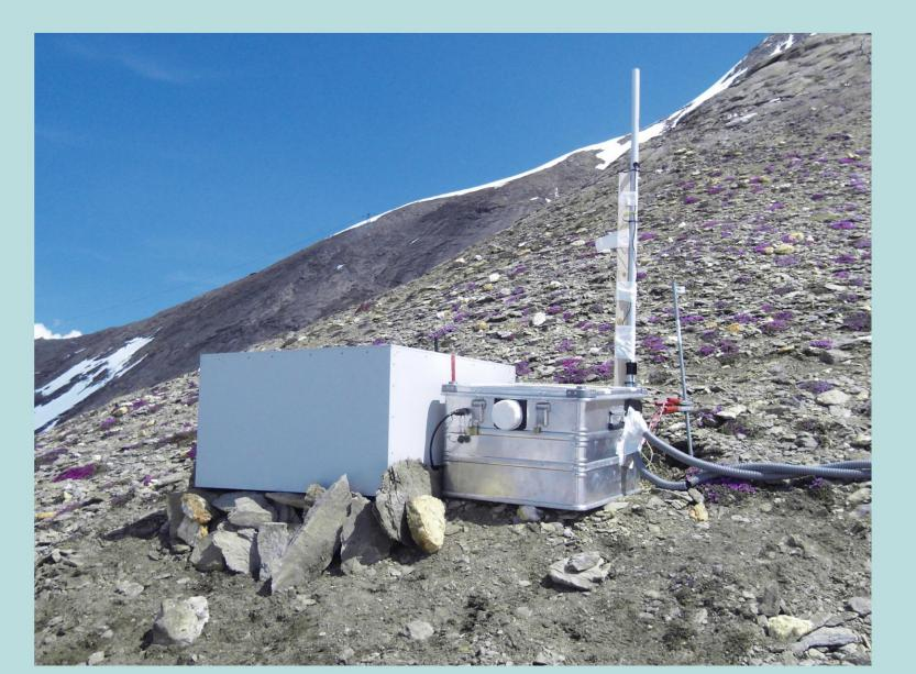
Fig.4: Due to the exposed position snow was blown into the instruments and power supply -> Box-in-Box solution
