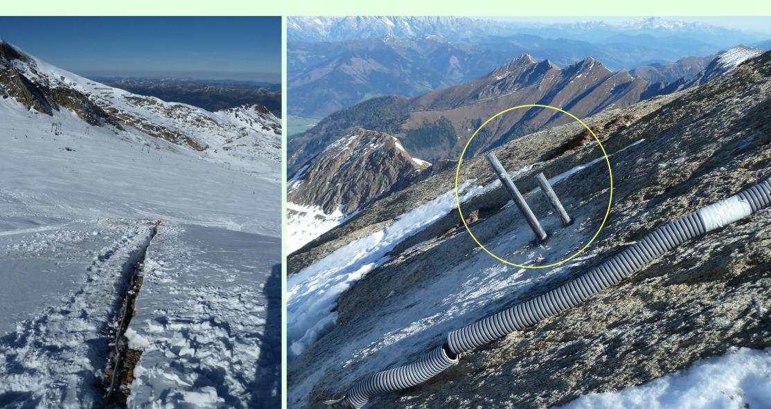
Fig.3: View of the monitoring profile (left, midle) and measuring point - rock temperature (right)
